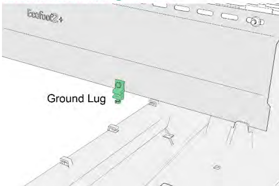
Ground hole with Lug Installed
